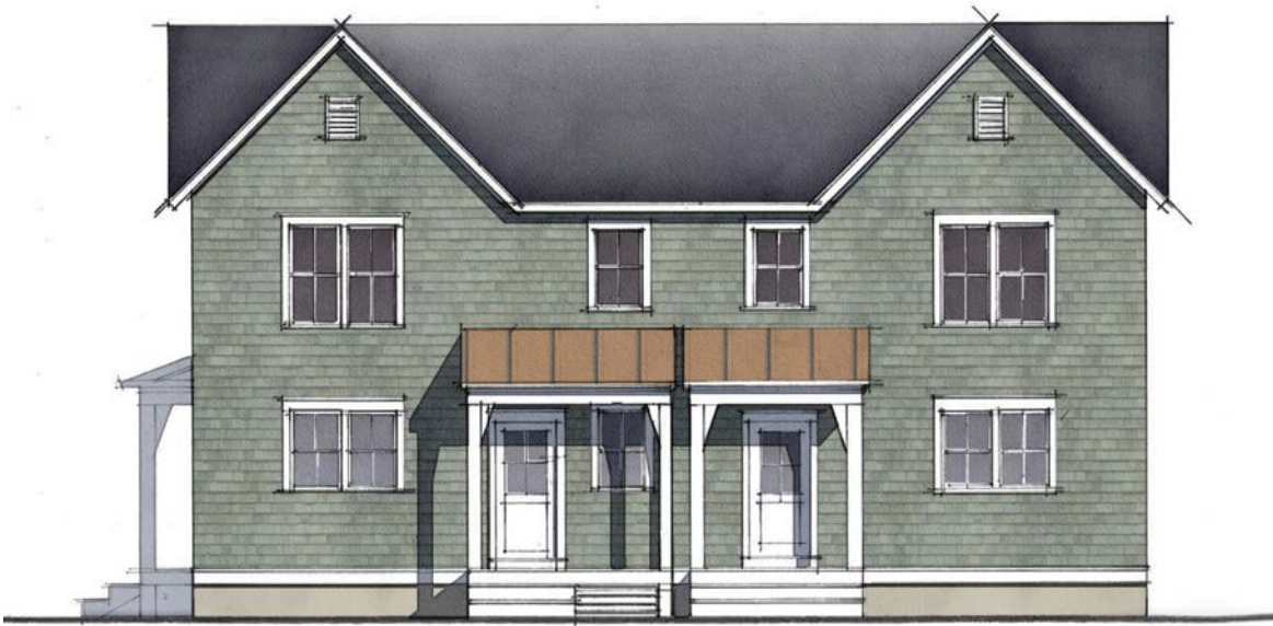
DUPLEX H-I REAR ELEVATION
