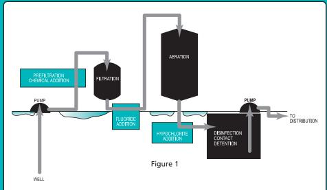
from the water. This aeration process removes the acidity from the water. The water is fluoridated and finally the water is disinfected with hypochlorite and detained in large holding tanks prior to being pumped into the distribution system.
