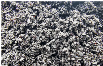
Ion Exchange Resin that has absorbed PFAS contaminants
